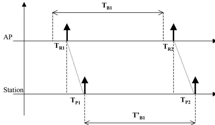
**Figure 3: Relation between beacon transmission and reception**
