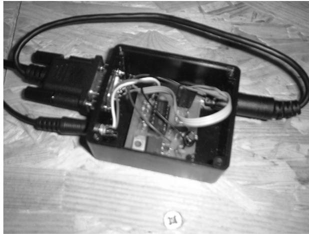
*Fig.3: Picture of the RS232-to-IrDA Converter*
