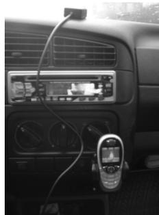
*Fig.4: Picture of the GPS mouse as connected to the phone*
