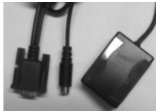
*Fig.2: Picture of the GPS mouse HI-201E used in our experiments*
