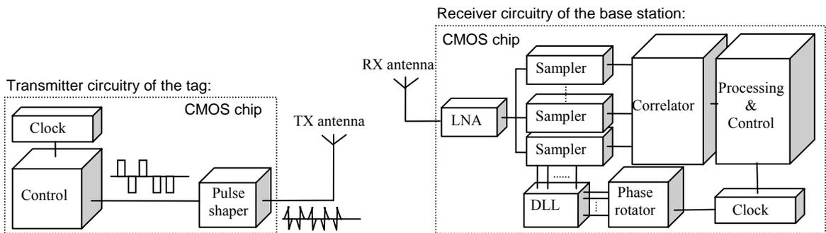
Figure 2: Basic building blocks of the tag's transmitter and the base station's receiver circuitry.
