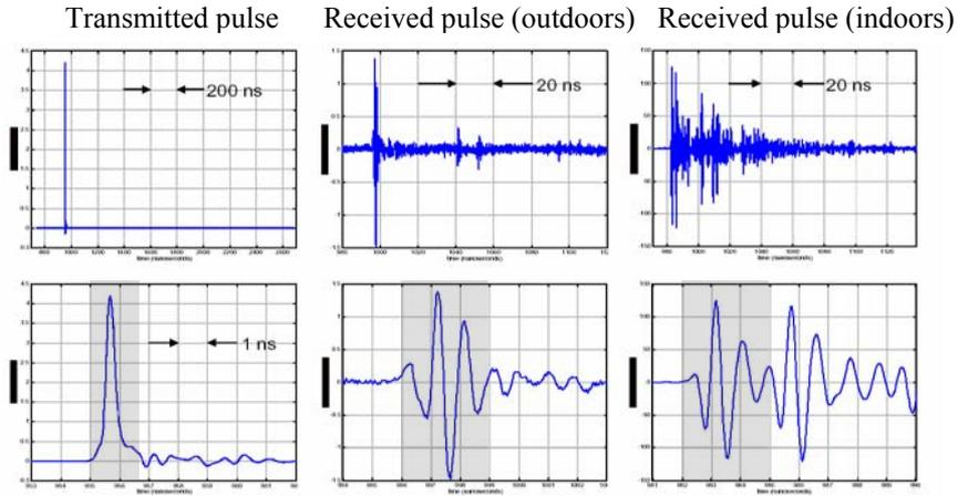
**Figure 3: Examples of UWB pulse transmissions under LOS conditions indoors and outdoors.**
