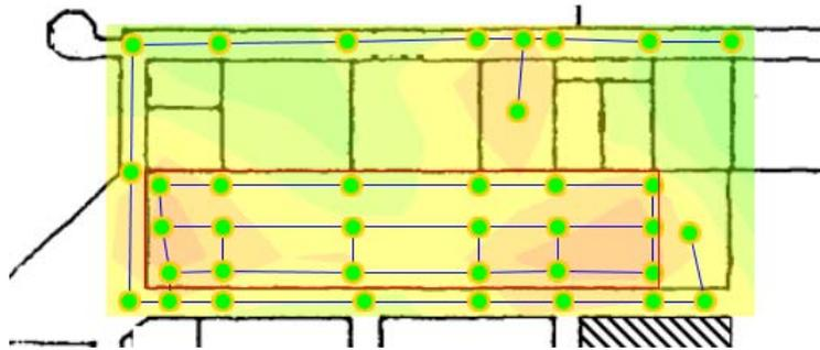
**Fig. 1** Ground plan of test environment with rails, calibration sites and isometric RSSI depiction.
