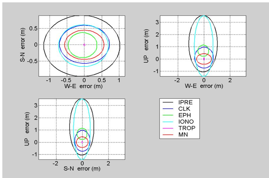
**Fig. 6: Repartition of  $2\sigma$  error envelopes at obe2.**
