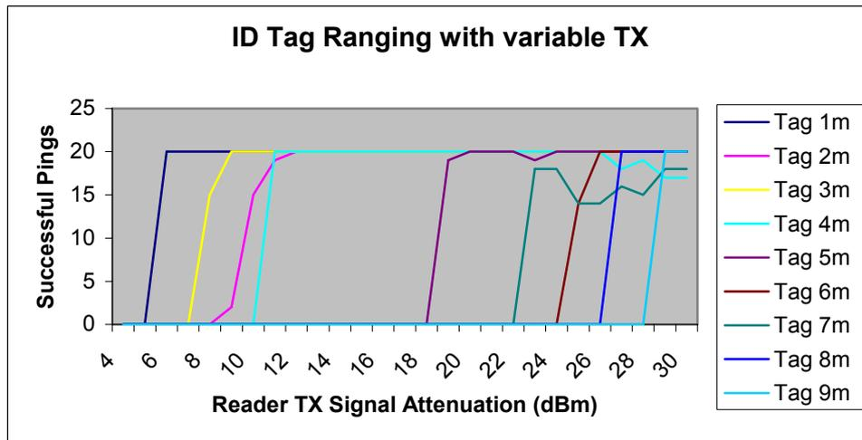
Figure 3 Room based short range RFID ranging
