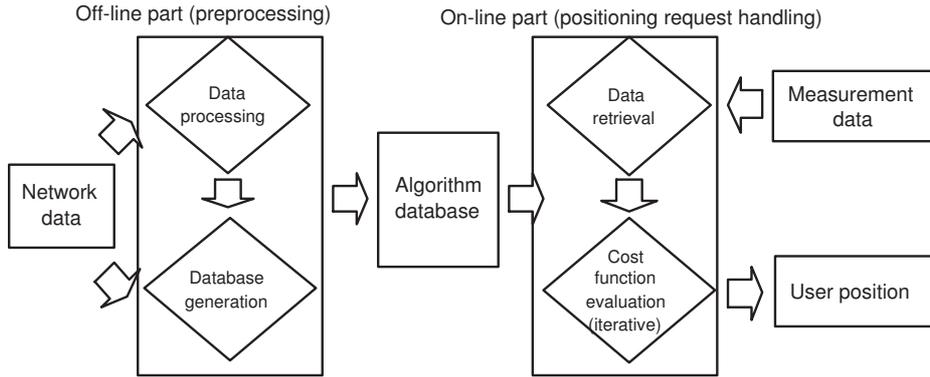
Figure 1: Positioning process flowchart
