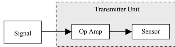
**Fig. 2.a Transmitter block diagram**
