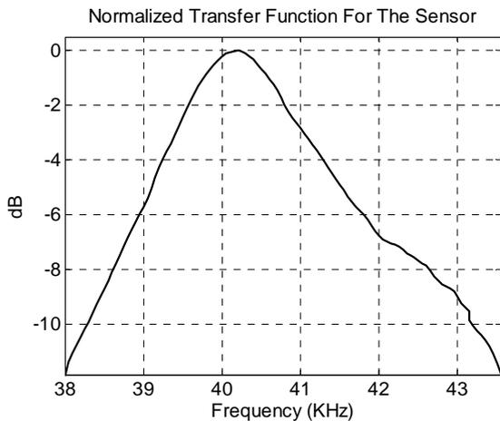
**Fig. 1 Normalized transfer function of the ultrasonic sensor**
