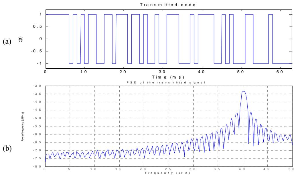
**Fig.3 (a) The transmitted code (b) the PSD of the transmitted signal**
