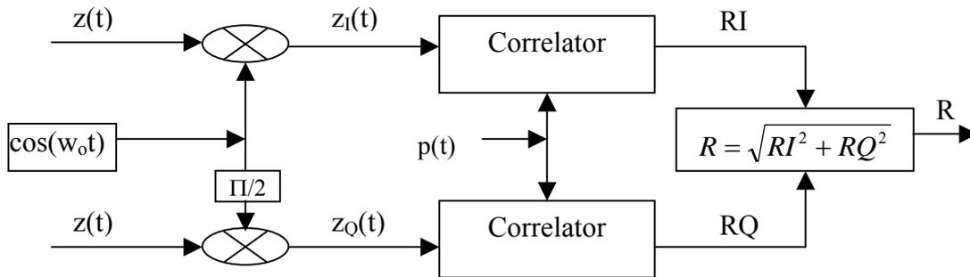
**Fig. 4 Two Channel Correlator Receiver.**
