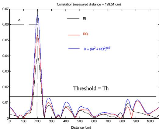
**Fig. 5 The correlation for the measured signal at distance (200 cm).**
