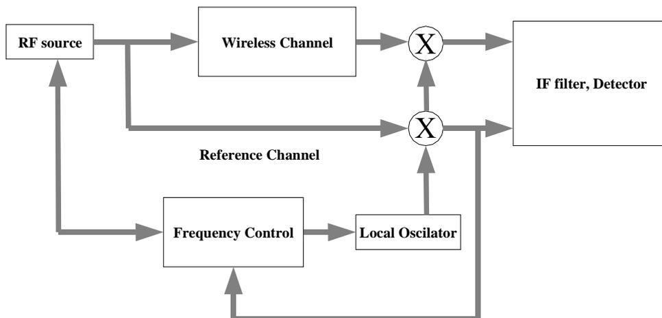
**Fig. 7 Schematic diagram of the transmitted reference VNA**
