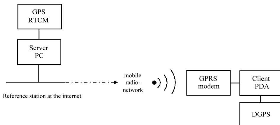
**Fig. 1 RTCM data stream on the Internet.**
