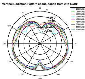
Figure 3b. Vertical radiation patterns of the disccone antenna at sub-bands
