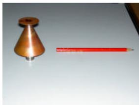
Figure 2c. UWB-Disccone Antenna
