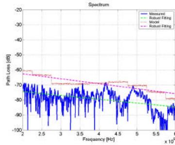
Figure 10b. Measured and simulated transfer function with a robust fitting of the power decay
