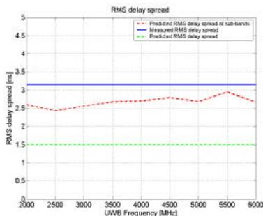
Figure 7b. Predicted and measured RMS delay spread over the sub-band
