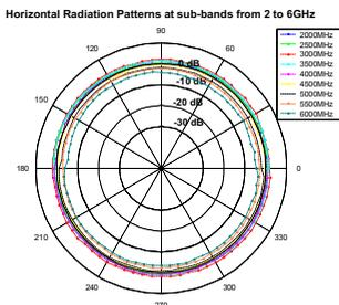
Figure 3a. Horizontal radiation patterns of the disccone antenna at sub-bands
