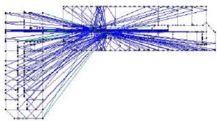
Figure 5d. 2D View of LOS simulation in the room A6-207 with up to 2<sup>nd</sup> reflection order
