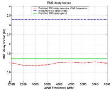
Figure 9b. Predicted RMS delay spread over the sub-bands
