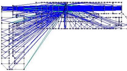
Figure 5a. 2D View of LOS simulation in the room A6-207 with up to 2<sup>nd</sup> reflection order
