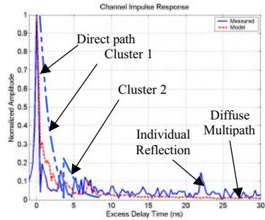
**Figure 6b. Measured and simulated channel impulse response for LOS**
