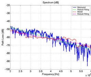
**Figure 6a. Measured and simulated transfer function in frequency domain with a robust fitting of the power decay factor**
