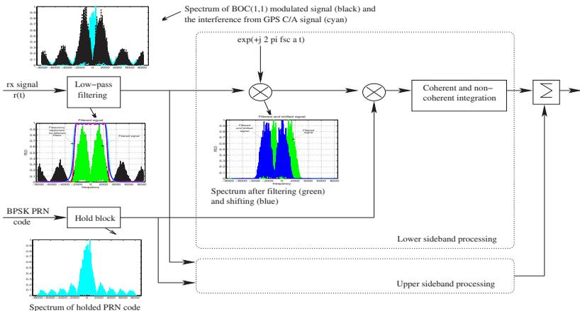
Figure 1: Block diagram of unambiguous proposed method (modified Martin & Heiries), dual sideband processing, even BOC modulation order  $N_{BOC}=2$ .
