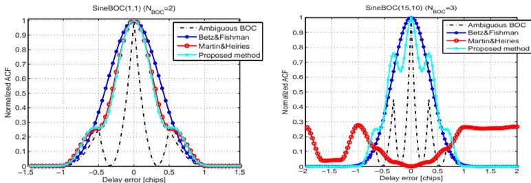
Figure 2: Illustration of the envelope of the correlation functions: **Left plot**, even BOC order,  $N_{BOC}=2$ , DSB processing, **Right plot**, odd BOC order,  $N_{BOC}=3$ , SSB processing. The ambiguous BOC shape is also shown as a reference.
