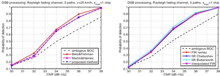
Figure 5: **Left plot:** Performance for different unambiguous methods, DSB processing, Rayleigh fading channel, 3 paths, sideband selection with IFIR filter, 2.046 MHz bandwidth, 0.0058 passband ripple and 0.1 stopband ripple; **Right plot:** Performance for different filtering structures used in sideband selection, DSB processing, SinBOC(1,1), Rayleigh channel, 3 paths,  $\Delta t_{bin}=0.5$  chips, sideband selection filtering is realized with the proposed low-complexity method
