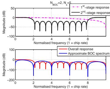
Figure 3: Frequency response of the two-stage interpolated FIR filter.
