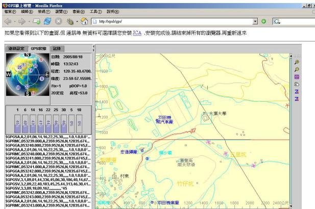
Fig. 3 The screenshot of execution. The satellite signals and data transmission status is on the left side; the map and trace are on the right side.
