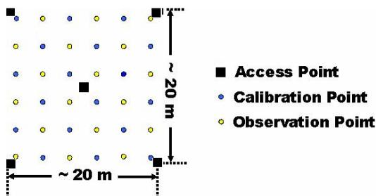
Fig. 4 Arrangement of access points, calibration points and observation points in the hangar environment
