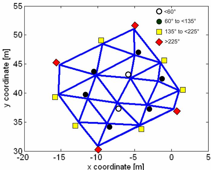
Fig. 3 Delaunay triangulation of calibration points and classification of maximal angles
