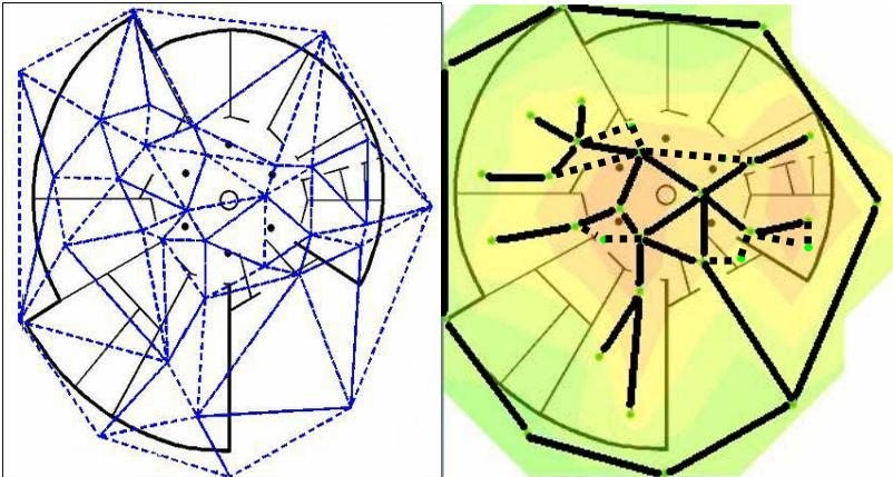
**Fig. 5 Unfavourable Delaunay trinangulation in the office building (left) and the remedy (right): usage of the EPE paths combined with additional lines**
