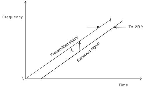
Fig.2 FMCW Radar frequency-time relationship
