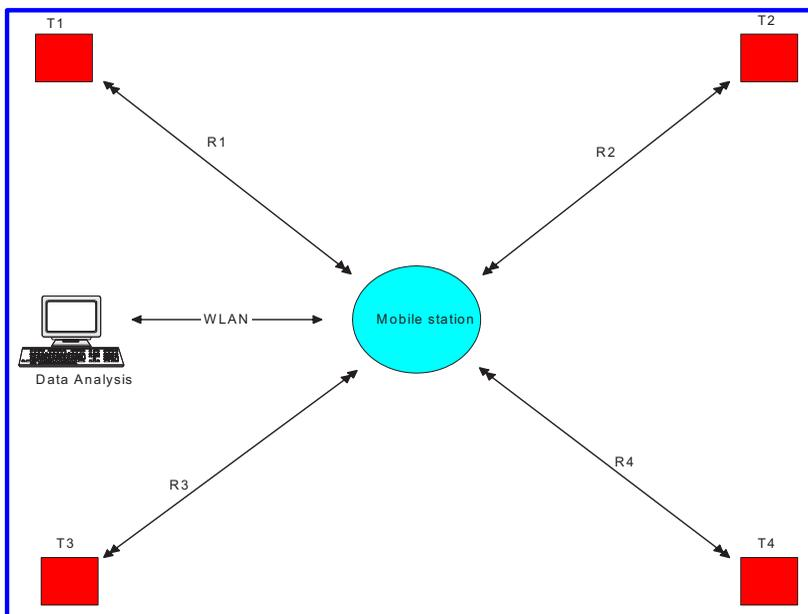
Figure (1): Plot of the measurement system with transponders and mobile station
