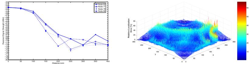
Figure 3: a) Averaged RSSI-curves for all four test nodes in the meeting room of our institute; b) Relative localization error [%] over a sensor field implying premeasured RSS-characteristics; algorithm: WCL, fieldsize:  $300 \times 300$ ; beacons 4; testpoints:  $300 \times 300$
