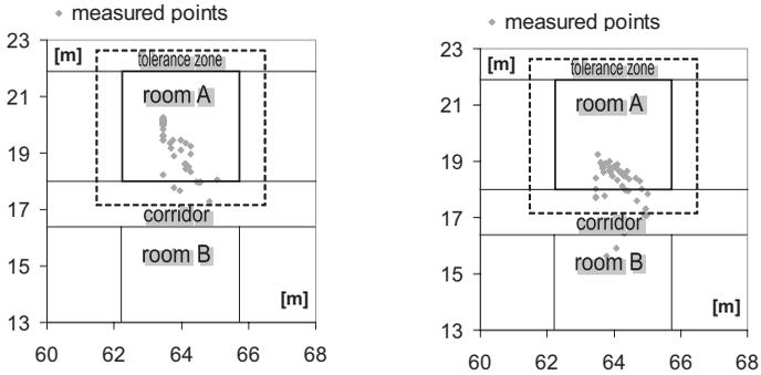
**Fig 6** Position fixes of a moving user in room A using one (left) or two (right) calibration points inside the room
