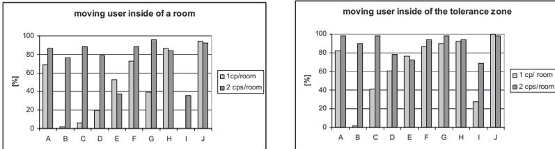
**Fig 7** Position fixes of a moving user inside a room (left) or tolerance zone (right) where one or two calibration points (cps) are used
