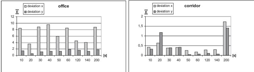
Fig 5 Standard deviations in x- and y-coordinates for calibration measurements with a duration of 10 s, 20 s, 30 s, 40 s, 50 s, 60 s, 1 min 20 s, 1 min 40 s, 2 min in an office room (left) and the foyer (right)
