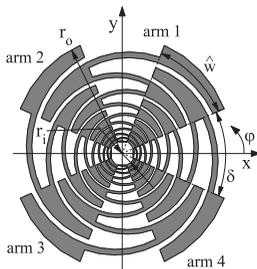
Figure 1: Geometry of polarization-diversity UWB trapezoid antenna in free-space.
