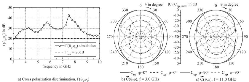
Figure 2: Simulated results for cross-polarization discrimination  $\Gamma(\vartheta, \varphi)$  and radiation pattern  $\bar{C}(\vartheta, \varphi)$  of UWB antenna design in free-space.
