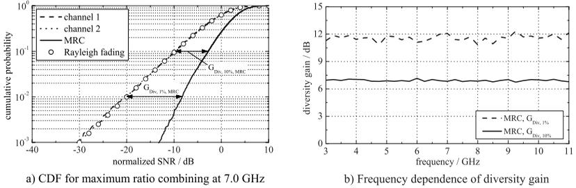
Figure 4: Results of polarization diversity performance for the UWB trapezoid antenna using maximum ratio combining.
