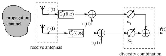
Figure 3: Model of receiver structure applying co-located, dual-polarized antenna elements and subsequent diversity combination.
